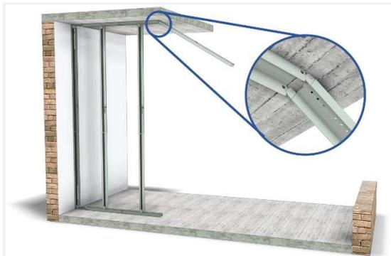
Click the large 120 cm door profile (= 2 I-modules) into the I-modules and fix it.
