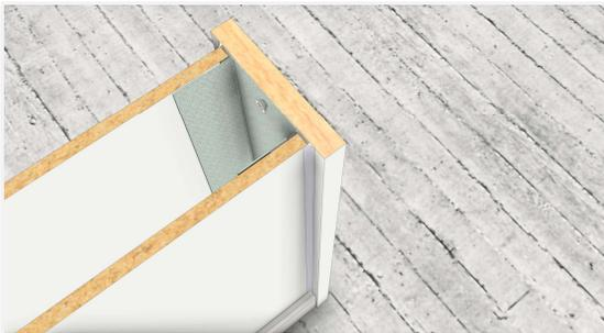
Finish off the joint between the click panel and end bar with sanitary silicone sealant.
