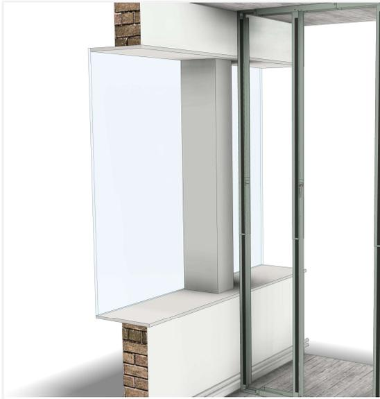
Fix the C-module as close to the window as possible.
