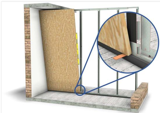
Place the wooden board on the shadow gap and level the board using shims. Then press the panel against the modules.
