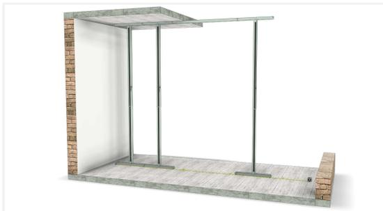
Insert the I-modules. Insert a door top profile in the place of the door opening.
