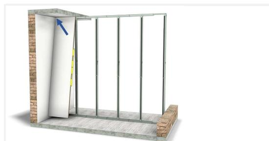
Install the first panel against the left wall and ceiling. Do not press the panel against the tape yet.
