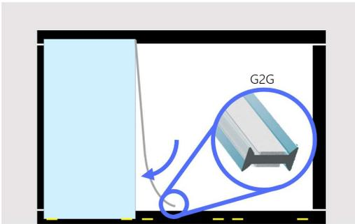
Remove dust and grease from the glass edge. Apply the G2G (Glass to Glass). Press firmly.
