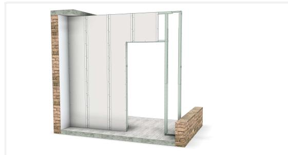
Screw the plasterboards to the structure using self-drilling screws. The drill point ensures that no collar forms around the holes. This increases the reusability of the modules.
