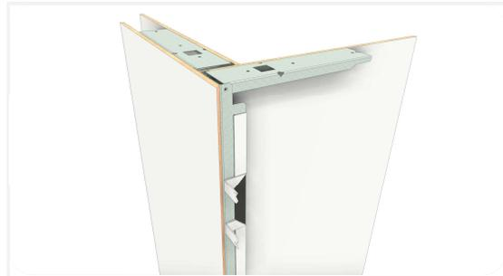
Apply JUUNOO tape (hook), pull the backing paper off, and degrease the panel on the back.
