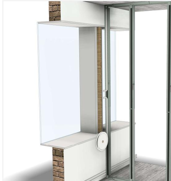
Fix a wooden bar to the window to support the click-in panel. Apply JUUNOO tape to the C-module.
