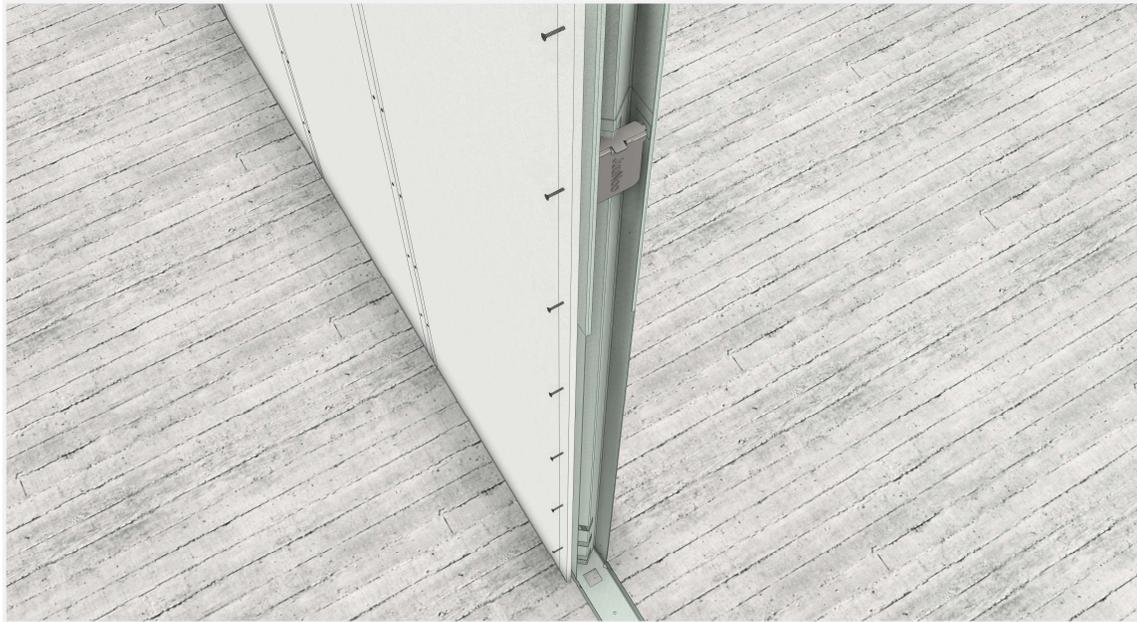
JUUNOO strongly recommends that you use a self-drilling version of these screws. This ensures that no lip is formed in the screw hole so that the profiles can continue to slide smoothly over each other after removal of the screw.
