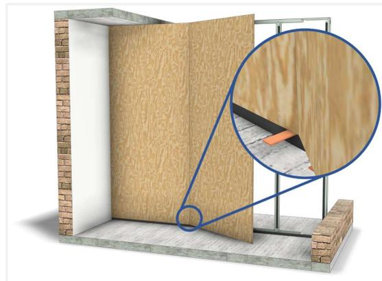
Leave the next panel hooked in to the first. Align the height with the first panel and rotate the panel to close it. Make sure the joint is firmly pressed shut.
