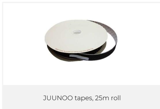
The JUUNOO tapes should be installed on a dust-free, degreased surface, at a temperature above 20 °C and at a humidity between 40% & 60%. After assembly, the JUUNOO tape must be pressed on firmly. The JUUNOO tape should be allowed to rest for at least 24 hours before loading.
