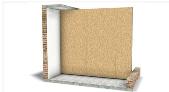
Finish the wall. Break off the shims under the panels, leaving a small piece under the panel. This ensures that the panel does not start to sag.
