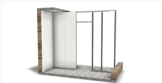
Mark the doorway on the back of the click panels. Do the same for each panel adjacent to the door. Saw off any excess. Make sure to leave a small gap between the panel and door frame (see below)
