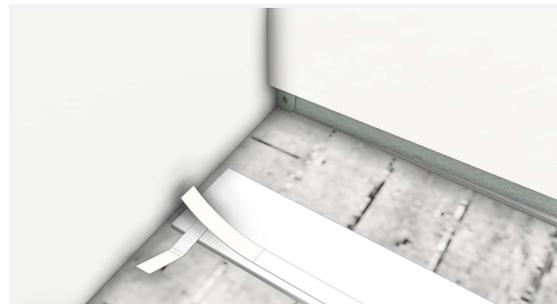
Insert a section of the textile tab under the tape. Make sure that the tab on the other side of the tape sticks out a little.
