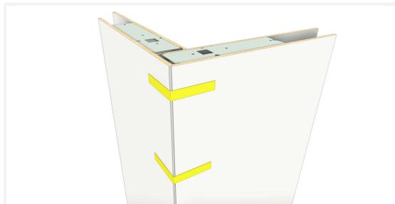
To allow it all to dry, clamp the 2 panels together using masking tape.
