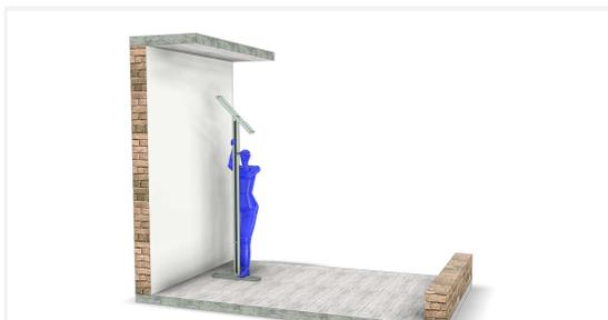
Open the Quickspan and slide the module open.
