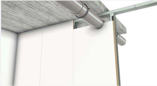
Without the pipe, the panel could rotate to snap into the 2<sup>nd</sup> panel. The pipe prevents this movement.
