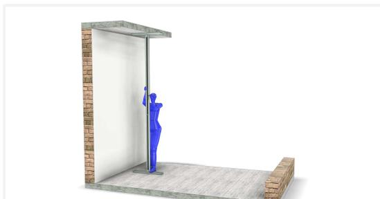
Clamp the module between the floor and ceiling by closing the Quickspan
