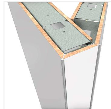
The construction of this corner is the combination of a 90° angle and a >90° angle. So, the effect is similar to both.
