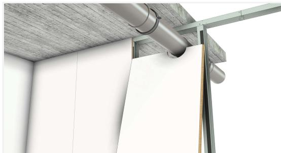
From the 3<sup>rd</sup> panel, make a cut-out for the pipe with a tolerance of 3 mm. Apply it from below, but do not press it against the tape of the I-module yet.
