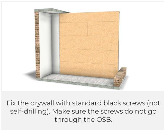
Fix the drywall with standard black screws (not self-drilling). Make sure the screws do not go through the OSB.
