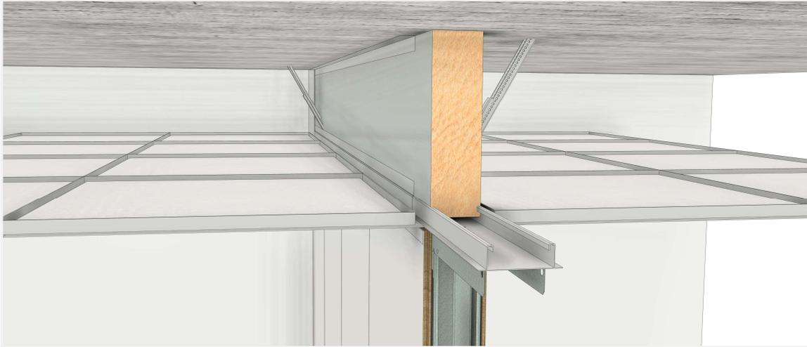
For an alternative arrangement, the drop ceiling can be installed after the installation of the JUUNOO wall. This is a more robust structure, but less easy to adapt.
