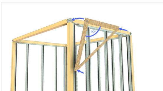
Temporarily brace the structure at right angles. Do this for each wall.
