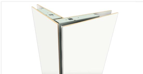
Fold the panel. Slide the profile leg between the already mounted panel and the C-module.
