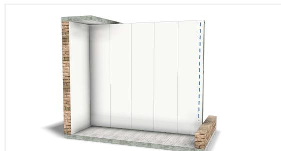
To dismantle the panels, use a multi-tool to saw off the edge of the last panel. The rest can be unscrewed.
