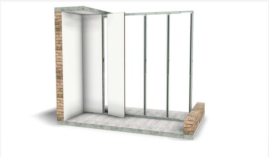
Apply the 2<sup>nd</sup> panel at an angle of  $\pm 30^\circ$ .
