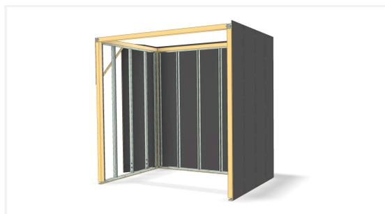
Attach the outer BaseClick panels to the modules. These will ensure the structure is rigid.
