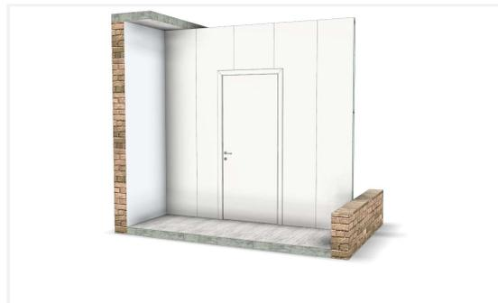
The architraves are prefabricated and cut to size. Attach them to the frame.
