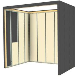
Place acoustic insulation between the modules.
