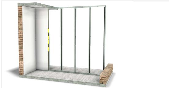
The panels are not placed directly on the floor to avoid possible problems with rising damp. Once level, press the panel firmly.
