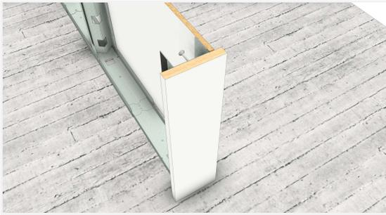
Leave at least one side of the module structure open, so that the bar can be fixed along the inside of the structure.
