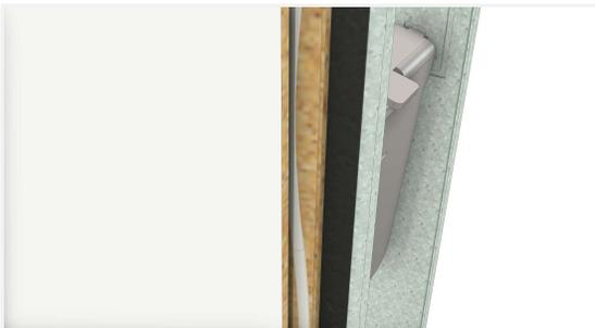
Apply a fine line of transparent silicone glue in the groove.
