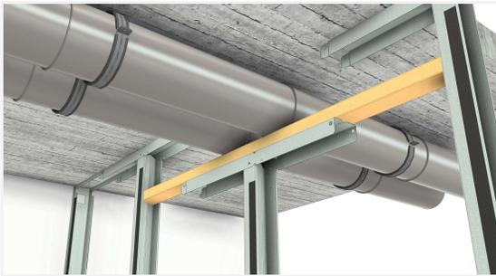
Position timber under the pipes and between the I-modules on the left and right of the central module.
