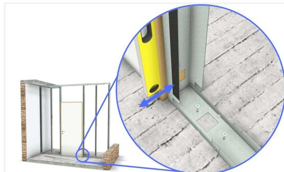
Level the bottom of the C-module on the hinge side and fix the base.
