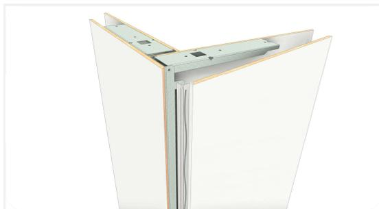
Apply sealant to the 'legs' of the corner profile, where there is contact with the panel. The profile does not need to be glued to the C-module.
