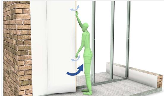
The tongue of the 2<sup>nd</sup> panel hooks into the groove of the first panel. Move back and forth until closed.
