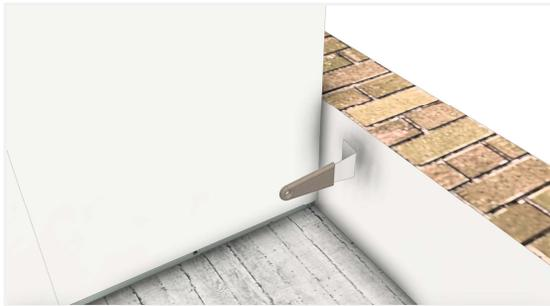
A putty or filling knife will be needed to loosen the JUUNOO tape between the first panel and the JUUNOO modules.
