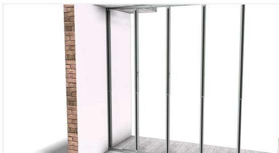
Click the C-module into the I-module at the top and fix into place.
