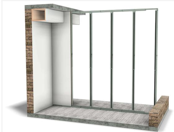
Fix the C-module bearing, cut I-module if necessary.
