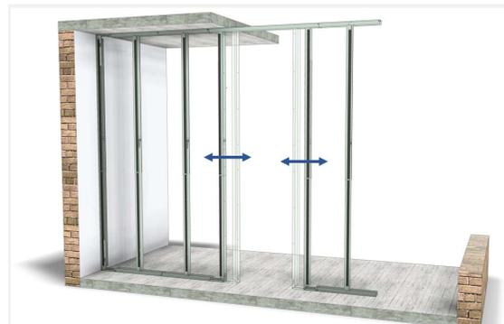
The placement of the C-modules/width of the door opening can be adjusted.
