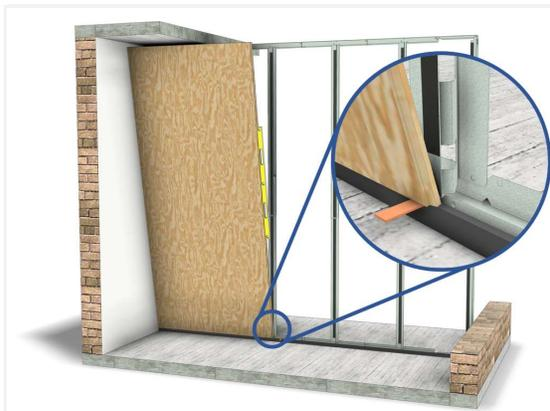
Place the panel with the groove against the wall on the shadow gap and level the board using shims. Then press the panel against the modules.
