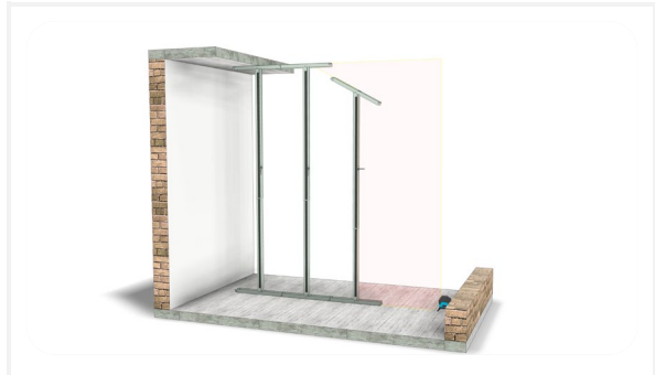
Continue this across the wall using I-modules.
