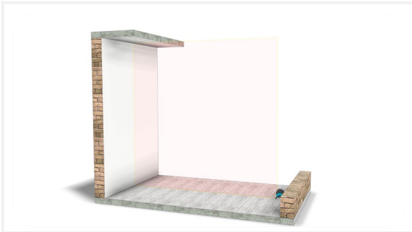
Place the laser on the centre of the wall.
